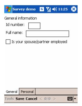
The main entry screen will appear, showing the design of the form, with the tabs and entry fields.
