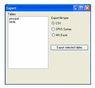
The name of the table to be exported will by default be the name of the file with a csv extension for CSV and xls for MS Excel. The exported files are stored in the same folder where the template was opened, which is also the one where the captured data is stored.
