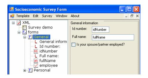
If you are entering data in the **idNumber** control, and you hit the Tab key, the cursor immediately jumps to the **fullName** capture control, as is specified in the left panel, *list of controls*. The order you see in the left panel is not necessarily the same as the one in the right panel, *view of controls*.
