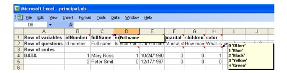
Notice that the first row is reserved for the name of the variable, and also includes the label of the variable in commentary mode. Row two shows the longer label of the variable. The third row includes the label of the codes for the definined variables (comboCtrl, radioCtrl and checkCtrl) visible as commentary. From the fourth row on you can see the captured values.
