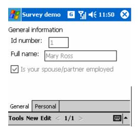
The lower menu has options from the menu and record navigation controls. The menu <New> prepares the screen for the entry of a new record and the menu <Edit> allows you to modify the current record.
