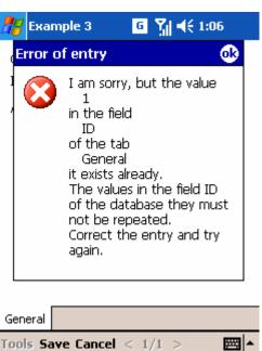
Also, since the attribute id='ID' is in place, the system established the ID field as the key field. If you try to add a value to the database which is already there, the system will not save the data. This way, values are not duplicated in the ID field.
