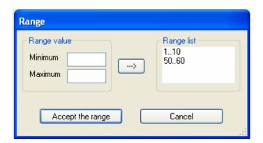
Fill out the **Minimum** and **Maximum** fields here with digits, and then press --> to add it to the range list, or select an item from the range list and then press <-- to
