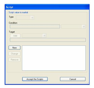
Firstly, to build the script click on *<New>*. Notice this enables the capture controls Type, Condition, and Target.
