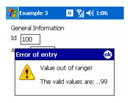
The numeric field is set to accept values at a range no higher than 99.
