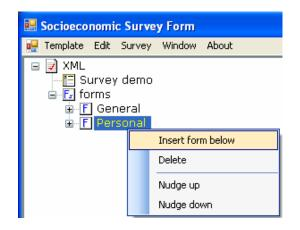
First we added the form by rightclicking on the last forms node, in this case the node *Personal*.
