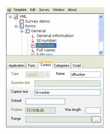
Some properties cannot be altered and that is why they appear in grey (disabled). The properties are disabled because they do not apply to this control. The user cannot modify the position control either as this has to be done in the control view with the mouse..
