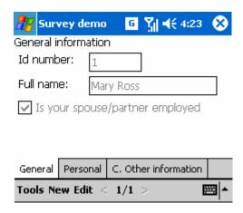
The screen appears divided in three tabs, as designed in the previous template. In the first tab (General) there are three filled fields and in the lower part of the screen you can find the 1/1 label that means that we are located in the first item of a total of one.
