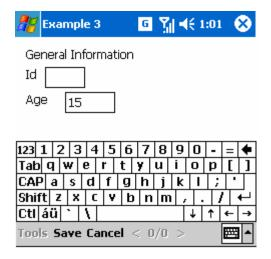
Example 3 shows a form with two numeric edition fields. Because of the autoKeyboard='True' attribute, by placing the cursor on any of the edit fields, the keyboard appears automatically on the screen. Note that in each new record, the name='age' field starts at 15 because it has been set to do so in the default attribute.
