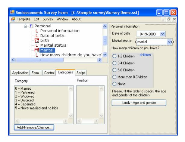
To add, delete, or change the entries of a *comboCtrl* or *radioCtrl* control, click on the button located in the lower part of the Categories tab. The dialog box *Category* will appear.
