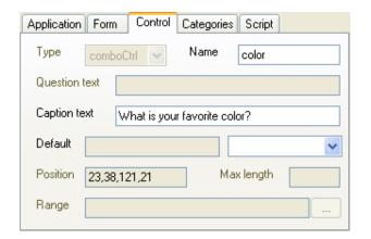
Notice that we have only changed the properties *Name* and *Caption text*. The property *Position* is readonly and its coordinates reflect the position the control occupies in the right panel *view of controls*.
