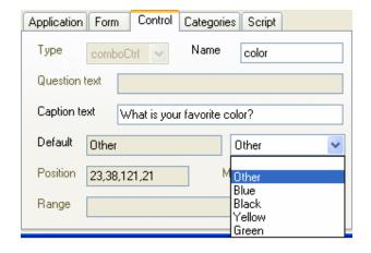
If you wish, you can give comboCtrl an initialization value so that it appears selected every time you capture a new record. In the Control tab click on the drop-down list located to the right of the property Default and select the initialization value.
