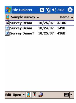
There are three files in the folder, one is the template that you used to capture data, and the other two are the XML files that contain the captured data. The data files are always going to have the name of the template, that is, *Survey Demo.xml* and *Survey DemoT.xml*. The first stores the data of the principal table and the second stores all the other tables that are generated (in this case only one table that is called *family*).
