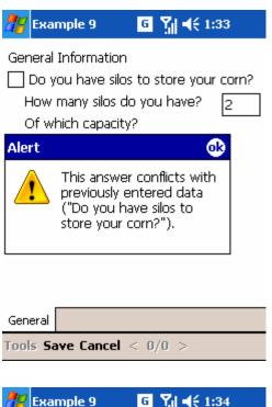
This example shows the use of the type="message" script. As shown in Example 9, if the question "Do you have silos to store corn?" is false and you try to enter an amount higher than zero, the question "How many silos do you have?" will display a warning message.
