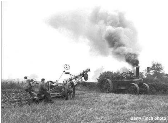
Fig.2- Fowler's traction engine pulling a plough (Source: Steam Plough Club, www.steamploughclub.org.uk/pictures.htm )
