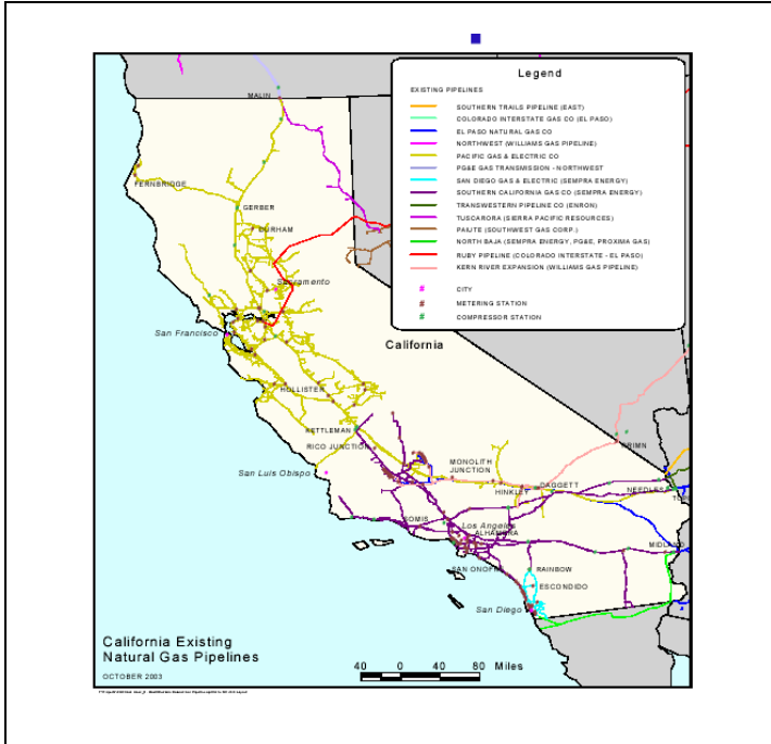
Figure 2: California existing natural gas pipelines and natural gas centers/hubs in relation to production basins and major flow corridors.
