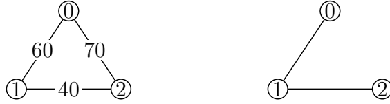
Figure 3.3: The optimistic mcst situation for \{1, 2\} (left side) and a related mcst (right side)
