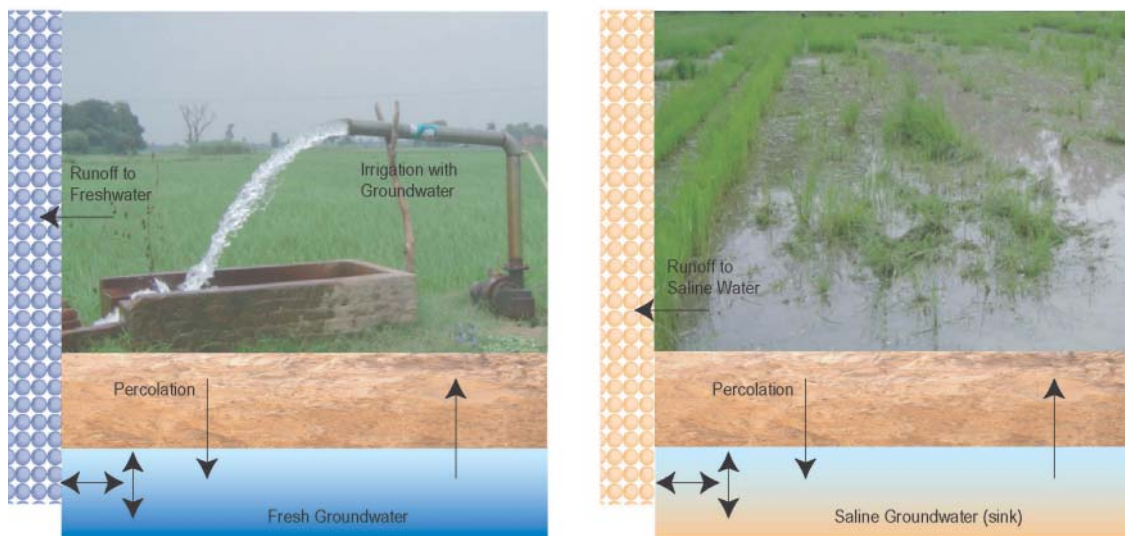
FIGURE 4. The interaction between recharge and abstraction of saline and fresh groundwater.
