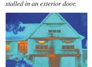
Once activated, the blower door pulls air out of the house. As air comes back into the house from elsewhere, Pace uses an infrared camera to essentially take an "X-ray" of the building and identify all the hidden air leaks and failed or missing insulation—the real causes for excessive energy usage and major comfort complaints. The entire process takes approximately two to three hours.
