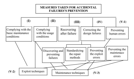
Figure 4 Measures of preventing the accidental failures
