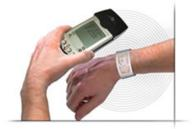
RFID tag draws power from this magnetic field and uses it to power the microchip's circuits. The chip then modulates the waves that the tag sends back to the reader, and the reader converts the new waves into digital data. RFID systems generally operate up to three feet at Radio Frequency or up to 20-25 feet at Ultra High Frequency. Possible issues surround eavesdropping, encryption, security, frequency and permissible error.
