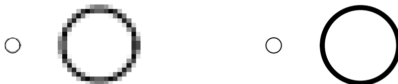
Figure 4: Two versions of a circle—a raster image (on the left) and a vector image (on the right)—at two different scales. Vector images scale better than raster images.
