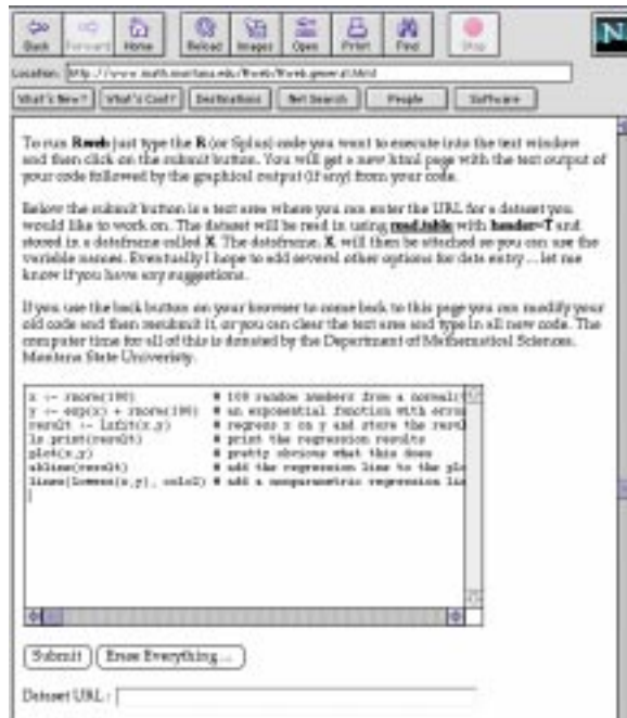
Figure 2: The basic Rweb page. The user types code into the text window then clicks on the submit button to have R execute the code.
