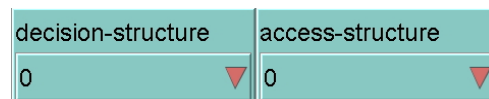
Figure 7. The buttons that select the decision structure (left) and the access structure (right). Non-segmented structures are denoted by 0, hierarchical structures are denoted by 1, specialized structures are denoted by 2
