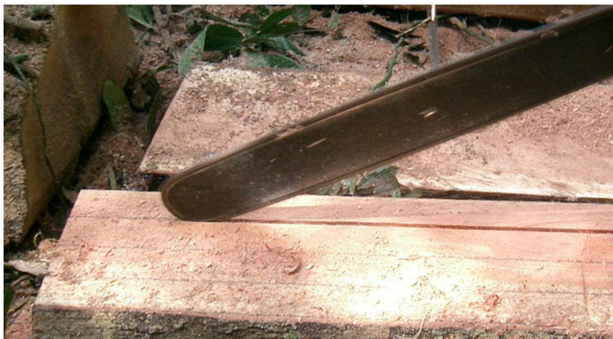
Fig 6 : Tracing the cut with the chain saw, following the tinted straight line (Photo R Nasi)
