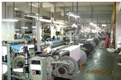
(3) Weaving the fabric on the weaving loom
