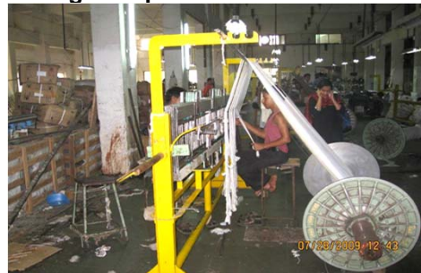
(2) Drawing the warp beam ready for weaving
