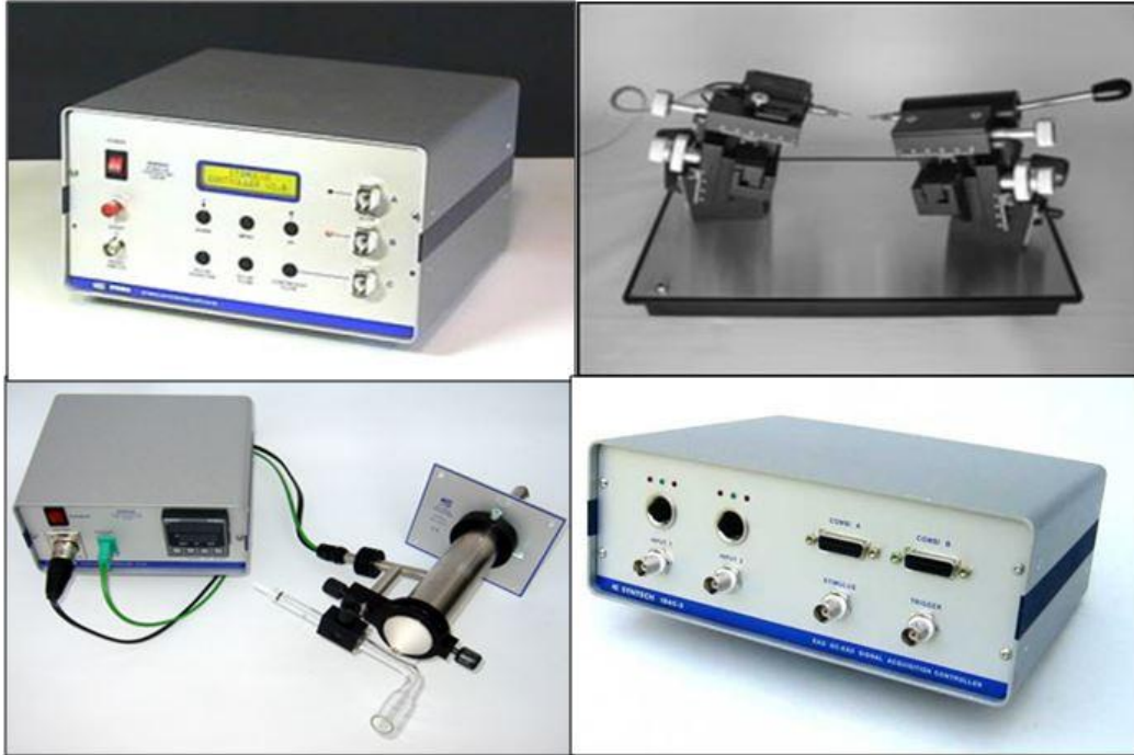
Figure 2. Electroantennogram (EAG) equipment. Top left: stimulus flow controller. Top right: 3 dimensional micromanipulators. Bottom left: continuous airflow tube connected to GC-EAD equipment. Bottom right: IDAC-2 high-impedance amplifier and two-channel controller (images from Syntech, Hilversum, Netherlands).
