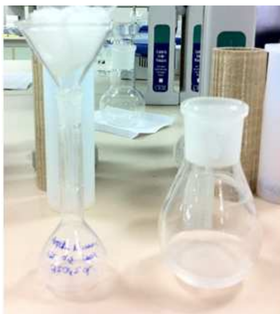
Figure 3.5 : Glass wool filtration.
