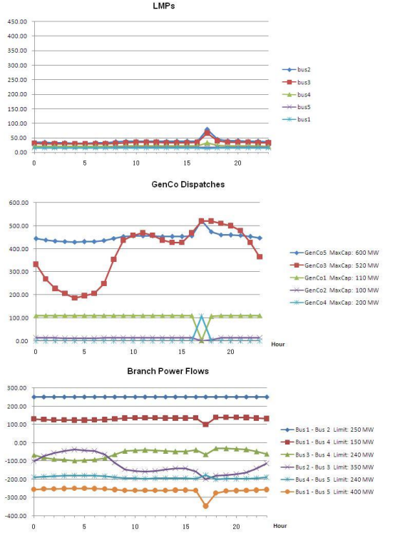
Fig. 13. Hourly bus LMP levels, GenCo dispatch levels, and branch power flows during a typical day for the benchmark dynamic 5-bus test case (no GenCo learning).
