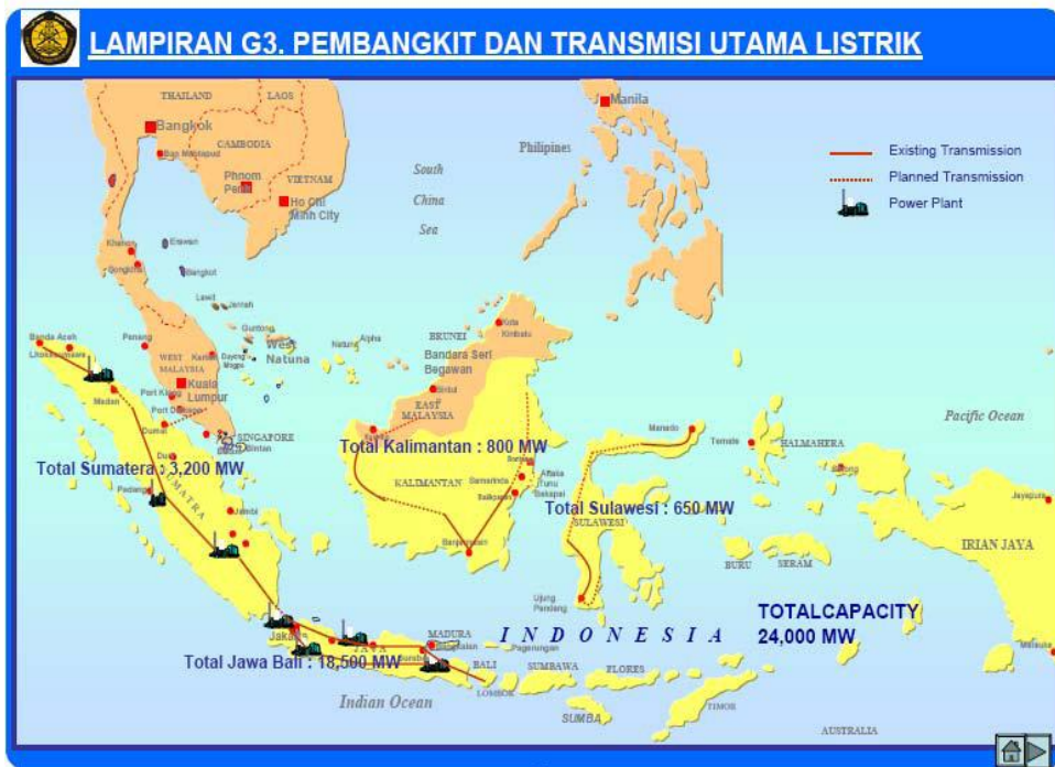
Figure 3.1 Indonesia Main Power Plants and Transmission Lines
