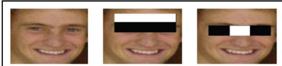
Figure 8: Examples of Haar features. Areas of white and black regions are multiplied by their respective weights and then summed in order to get the Haar feature value.
