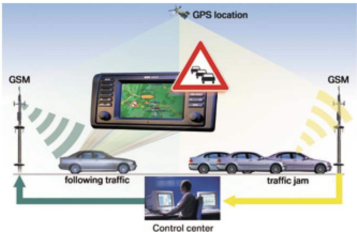
Figure 4.1 Floating car data mechanism demonstrated by BMW
