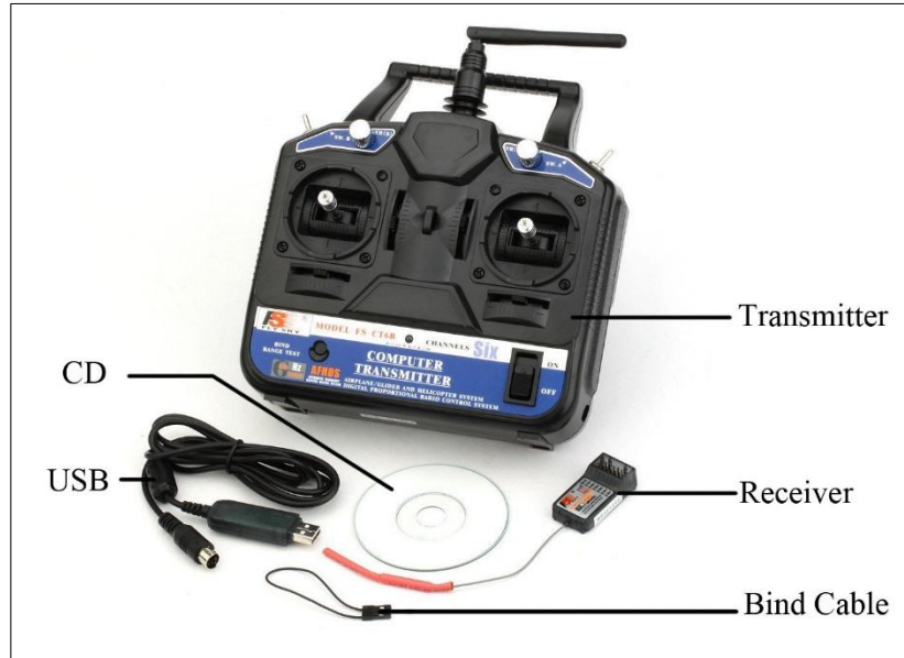
Figure 2.30 – FlySky 6 channel radio transmitter and receiver [19]
