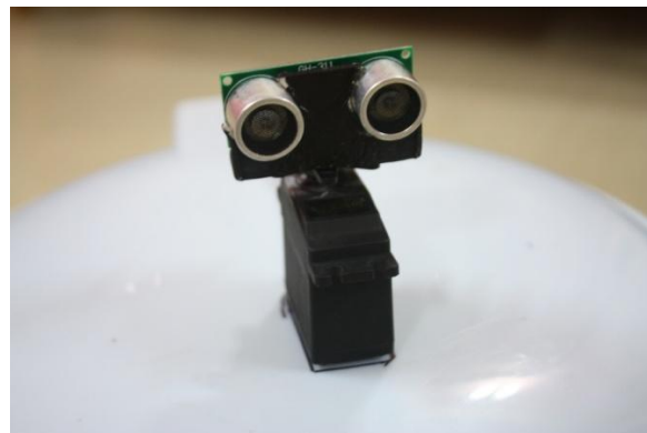
Figure 7: Ultrasonic sensor mounted on servo motor.
