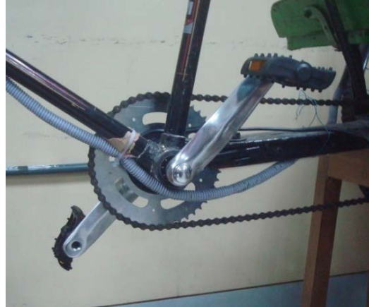
Fig. 6.4 The torque-sensor pedal assembled replacing the old pedal
