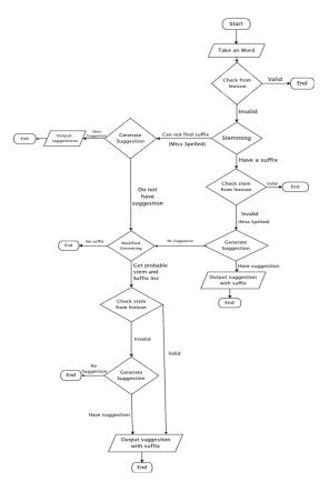
Fig 1: Flow chart of Spelling Check Algorithm
