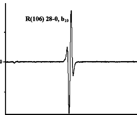
FIG. 4. Signal-to-noise ratio of R(106) 28-0, b_{10} sketched by our portable laser system. Time constant: 20 ms. Modulation width: 6 MHz.
