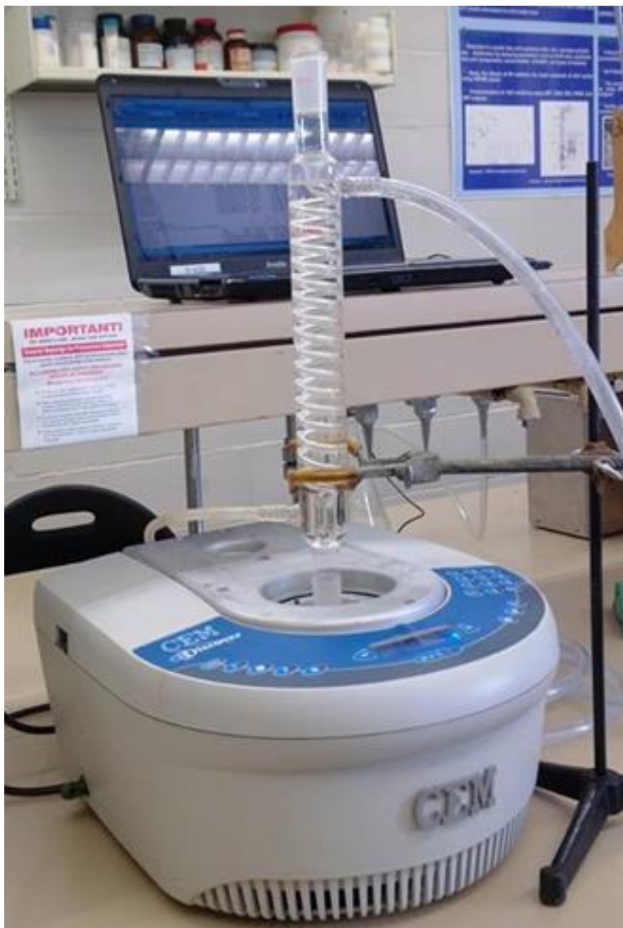
Figure 3-1. Photograph of the single mode microwave set-up used of Na-A zeolite under atmospheric condition
