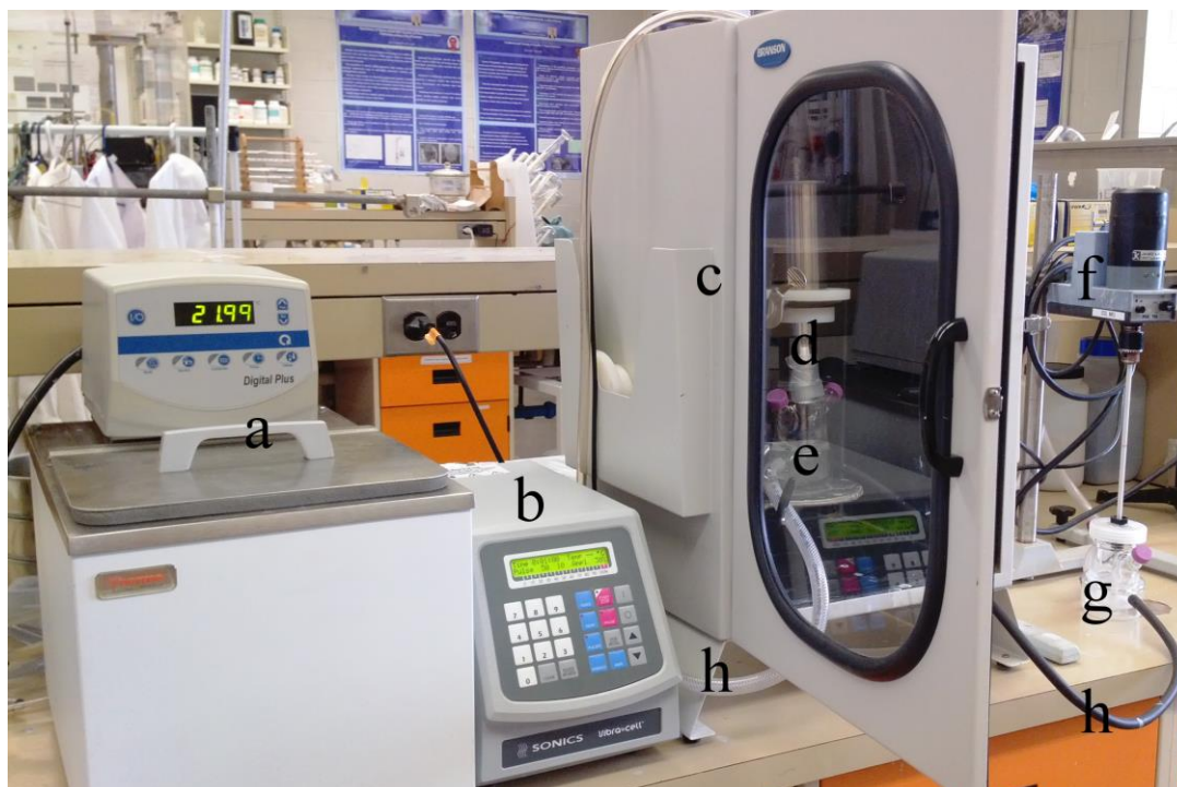
Figure 5-1. Photograph of the experimental setup used for reaction a) temperature control and water circulator b) 500 Watt ultrasonic processor c) noise cancellation box d) ultrasound probe e) crystallizer #1 with UTS assistance f) mixer g) crystallizer #2 conventional heating h) piping for temperature control water circulation
