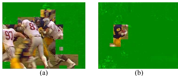
Fig. 3. Intra-coded blocks in the high-pass frame of the lowest temporal layer in (a) the third GOP (higher temporal activity) and (b) the eighth GOP (lower temporal activity) for Football .
