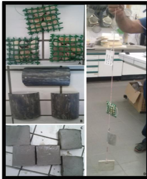
Figure 2.4 The three different material surface components used in the case study performed at the Olhão recreational port. A) Plastic grid wallet filled with stones, B) PVC surfaces, C) Cement plates and D) The final device with the 3 surface components and identification tag on the upper portion.
