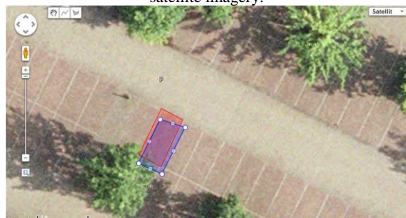
Figure 5: Translating the projection back to (geographic) world coordinates and projecting them back on the used satellite imagery.
