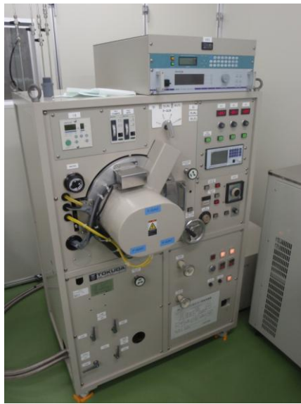
Fig. 3.5. A DC sputtering system.
