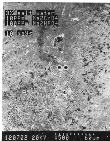
(e) 3% NaCl with 10 ppm \text{Na}_2\text{CrO}_4 and 100 ppm \text{Na}_2\text{HPO}_4
