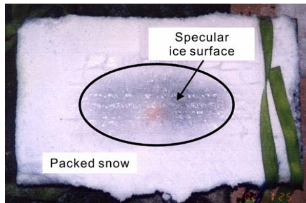
Photograph 1 Refreezing of packed snow surface after melting due to tire frictional heat associated with wheel slide. (number of passage of wheel = 5000, room air temperature = -3^{\circ}\text{C} )
