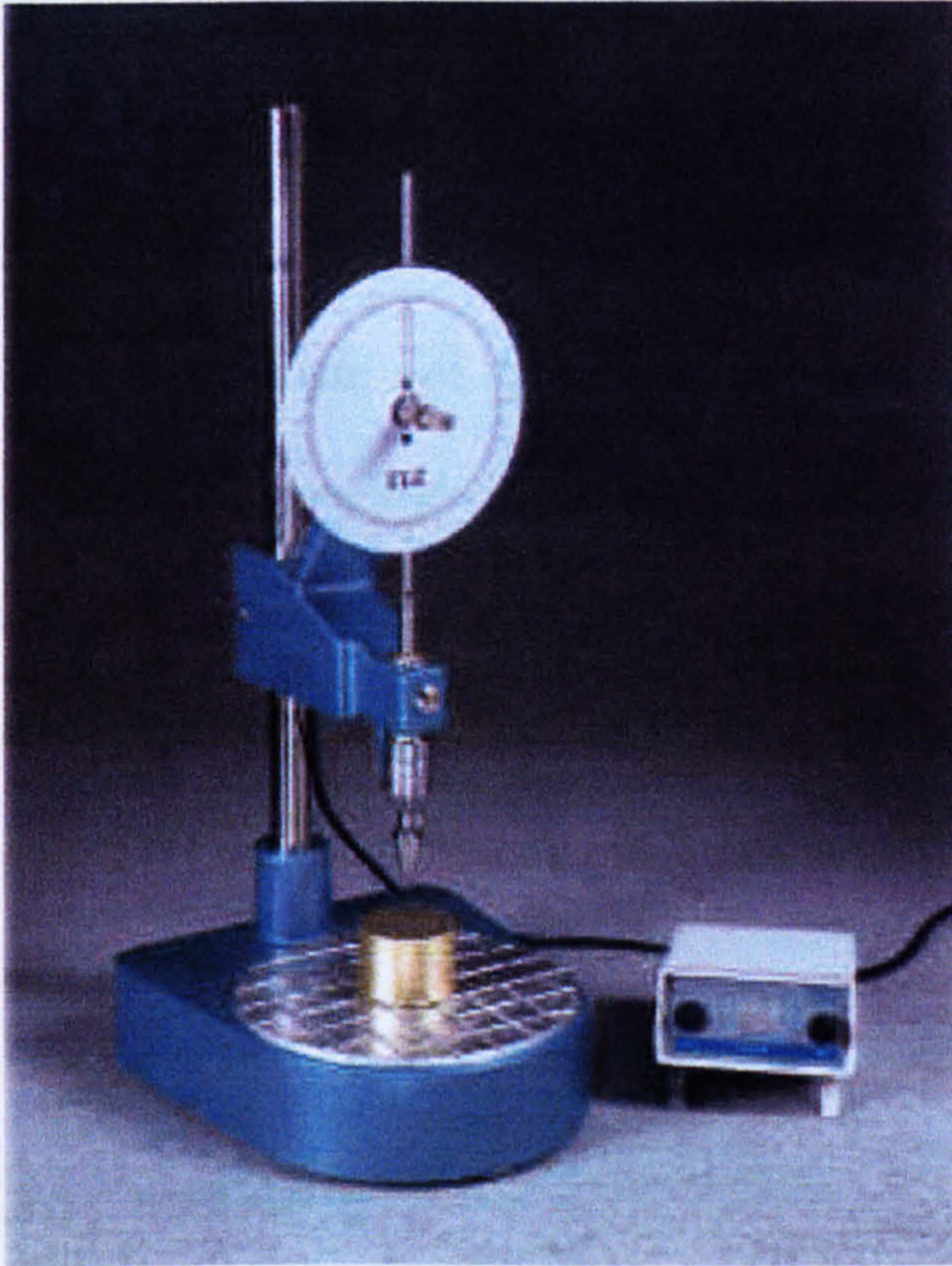
Plate 6.1 Falling cone penetrometer used in Atterberg (consistency) limits.
