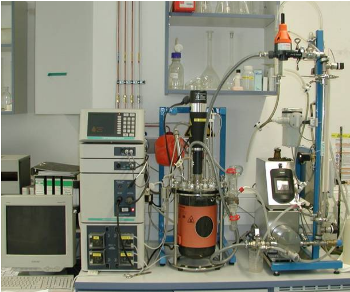
Figure 13 Set-up of the of the Anaerobic Membrane Bioreactor (AMR) at the Environmental Process Laboratory at the University of Applied Sciences and Arts Hanover in Germany.
