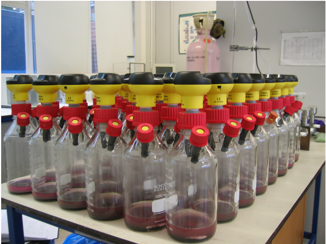
Figure 10 Test vessels containing inoculated samples, sealed and fitted with OXI-Top-C pressure measurement devices.
