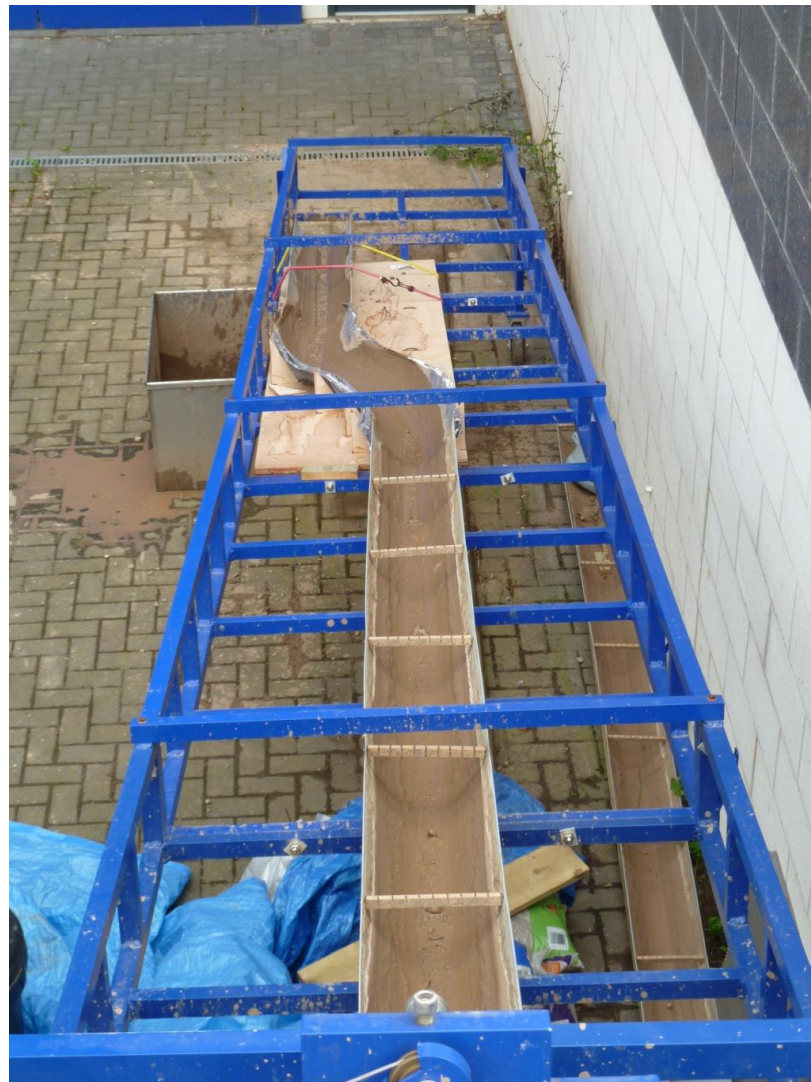
Figure 3.10: Channel bend inserted into the flume structure. The geometry of the channel bend is R_c = 0.7 m, \theta = 40^\circ
