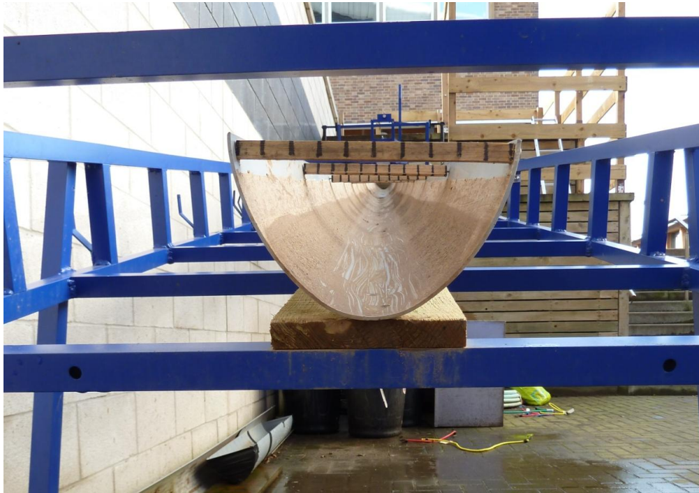
Figure 3.2: A cross section of the channel, demonstrating the parabolic shape. Note, wooden marker is 0.2 m across.
