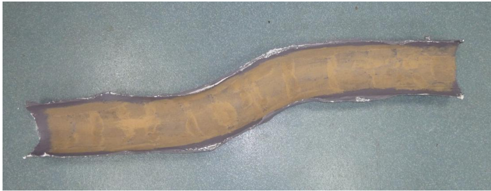
Figure 3.9: A completed bend having been reinforced, painted and a sand coating applied. Bend is R_c = 0.55 m, \theta = 40^\circ
