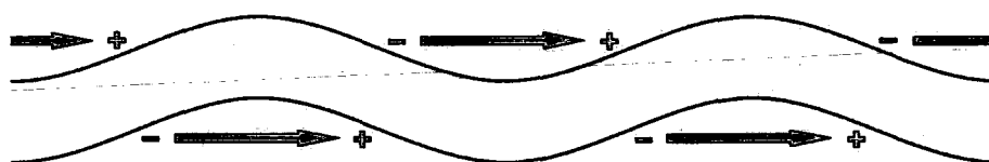
Figure 2-21: Conformal roughness across the barrier leads to so called orange-peel coupling of the electrodes through the barrier. The magnetic poles involved are shown by the + and - symbols on the figure.
