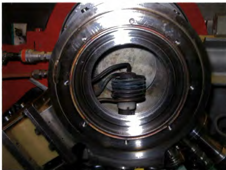
Figure 3-7: The furnace chamber with sample mounted in the centre. The RF induction coils are clearly visible around the sample stage and column.
