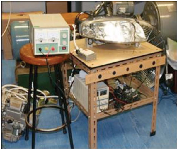
Fig. 17 Testing Platform of Low Beam Levelling System
