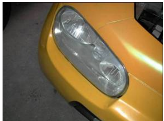
Figure 21 HID installed to the EV4.
