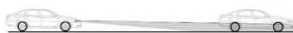
Figure 1 Vehicles sits horizontally – Light beams Since the headlamp is adjusted according to the horizontal level. The headlamp focuses positions correctly.
