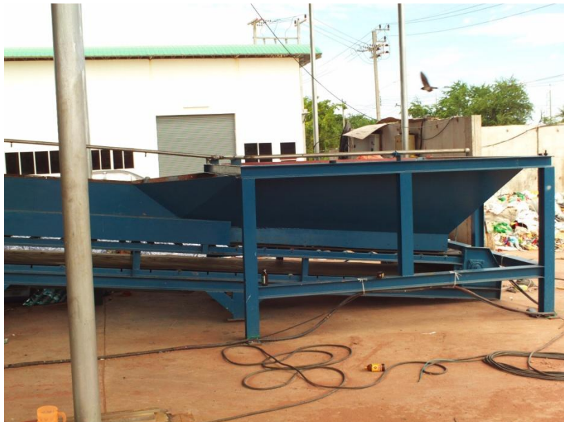
Figure A1-2: Feed Hopper
