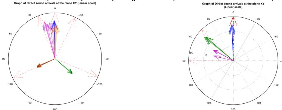
**Figure 1:** Repeatability of the Soundfield Microphone in Blue room 2 (Left graph) and Live room (Right graph). Left Front speaker and 90° position (Purple), Centre Front (Blue), Right Front (Light Brown), Left Rear (Dark Brown), Right Rear and 45° position (Green), Real directions (dashed lines)
