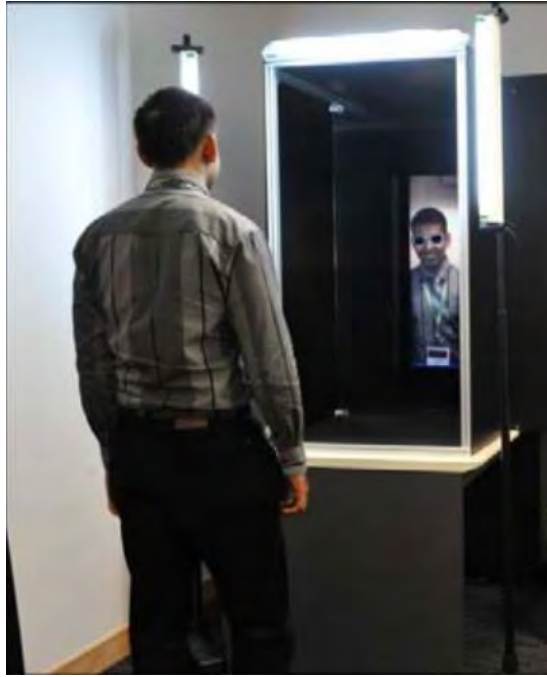
Figure 2.6. The 3D virtual eyeglasses try-on system (Yuan et al., 2011)
