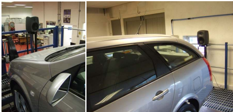
Figure 6 – Positioning of noise sources ahead and behind vehicle to generate road and background noise. Pink noise was being reproduced.
