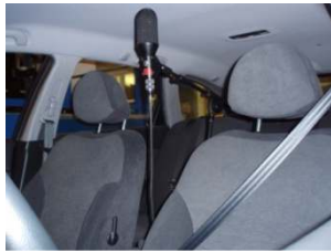
Figure 5 – Microphone placement inside the car and between the two front headrests. On-axis direction points straight ahead.
