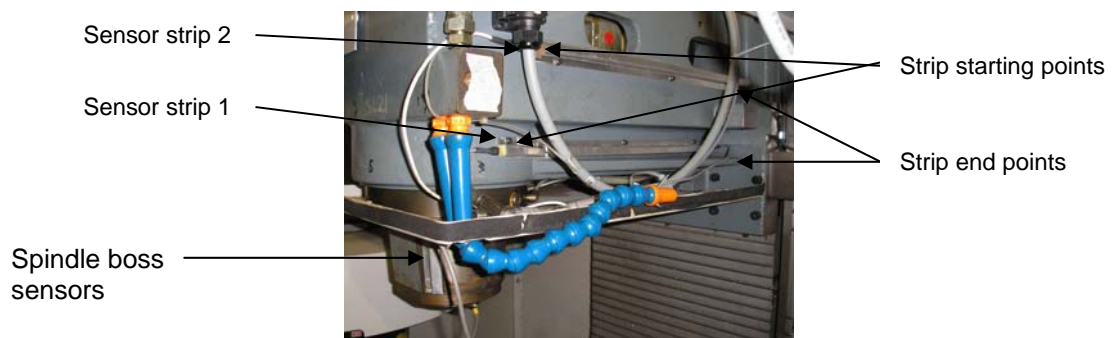
Figure 7: Thermal sensors location on the machine
