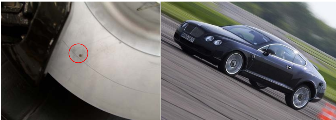
Figure 1: Thermocouple in Front Brake Disc and Test Vehicle Fitted with Slip Rings
