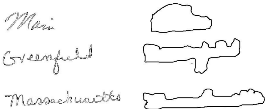
Figure 1.3: The word shape of cursive words alone contains sufficient information to classify the image as one of the lexicon words [1]
