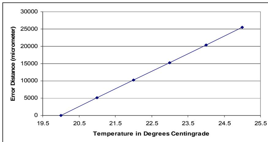
Fig. 6. Temperature versus Error Distance in dry air.
