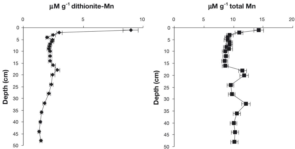
Fig. 10. Vertical profiles of dithionite-extractable and total Mn (HNO<sub>3</sub>/HCl/HF extraction) for Core LD1, Loch Duich. Mn determined by flame-atomic absorption spectrometry (Perkin Elmer 3300) following standard dithionite or HNO<sub>3</sub>/HCl/HF extraction (for details see Krom et al. 2002)
