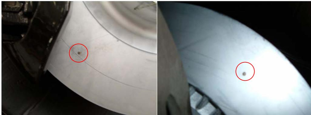
Figure 2: Position of Thermocouples in Front Brake Rotor
