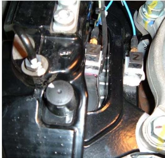
Figure 1: Caliper and back plate accelerometer positions
