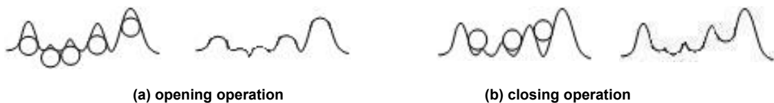
Fig 4: Examples of opening and closing operations in morphological processing
