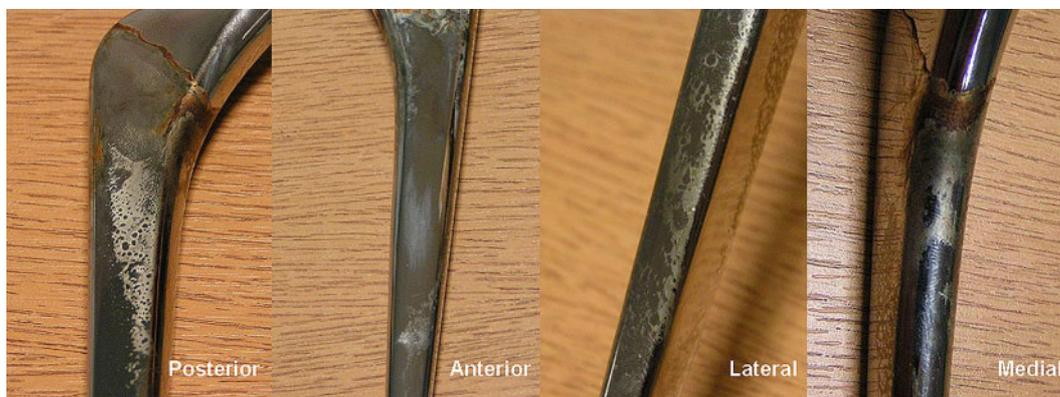
**Fig. 4** Fretting wear generated on the surface of an Exeter polished femoral stem through an *in-vitro* wear simulation
