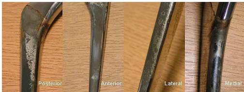
Figure 1: Reproduction of fretting wear on a polished Exeter stem
